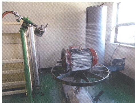
Photo 2-2 Test set-up for IPX4 (Model : AF3502)
