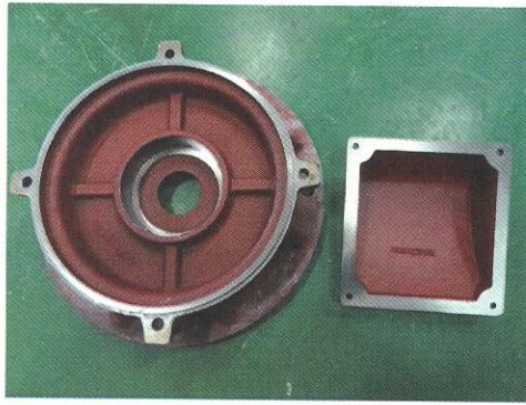
Photo 1-4 Test result for IP5X (Model : AF3502)
