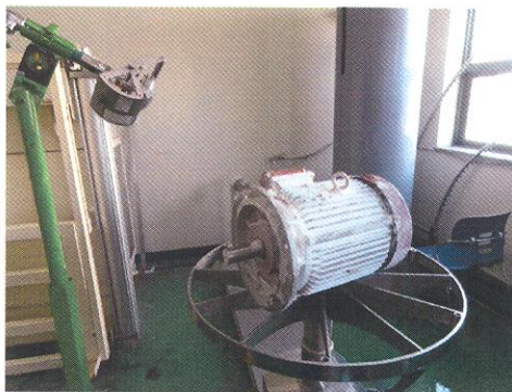
Photo 2-2 Test set-up for IPX4 (Model : AF3502)
