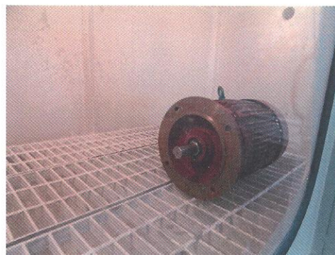
Photo 1-1 Test set-up for IP5X (Model : AF2152)
