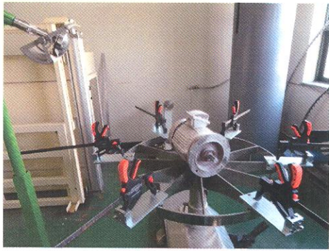
Photo 2-1 Test set-up for IPX4 (Model : AF2152)
