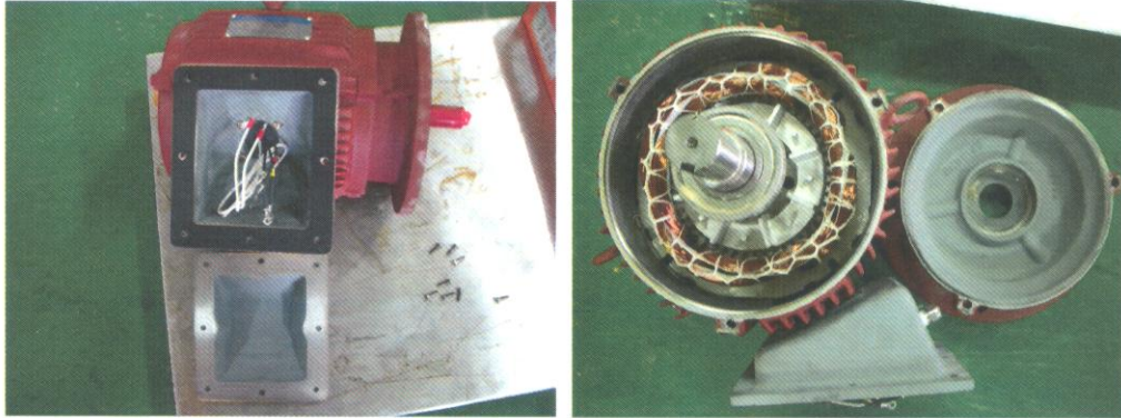
Photo 2-3 Test results for IPX6 (NF2155)
