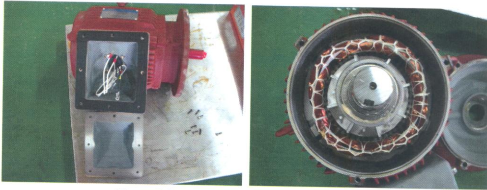
Photo 1-2 Test results for IP5X (NF2155)
