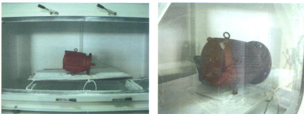
Photo 1-1 Test set-up for IP5X test
