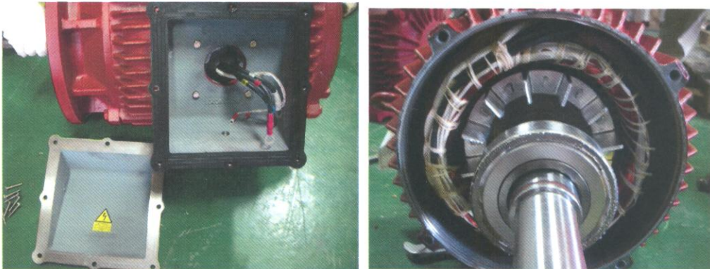
Photo 2-4 Test results for IPX6 (NF3005)
