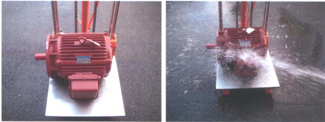
Photo 2-2 Test set-up for IPX6 test (NF3005)
